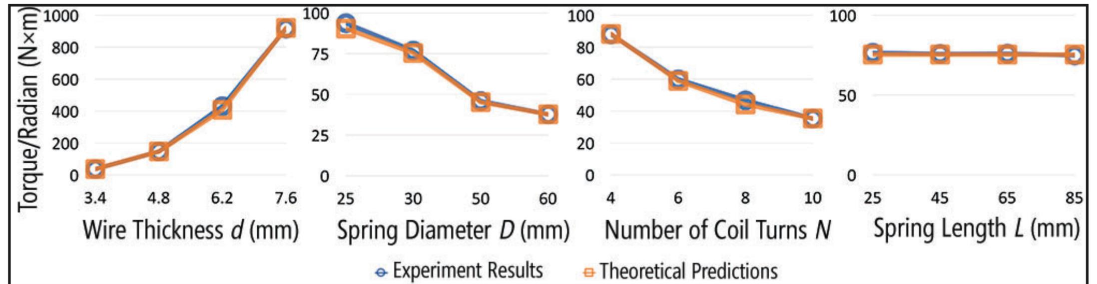
The tensile and torsion behaviors of 3D-printed helical springs closely mirror theoretical predictions
