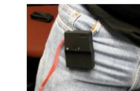
Figure 1 (left) The UbiGreen Transportation Display shows transit behavior as "wallpaper" on a phone's screen. Here the tree is nearly full of leaves, indicating that the user has completed several green trips for the week. (top) The MSP sensor worn near the waist and the phone's GSM cell tower data are used to semi-automatically infer transportation mode.
