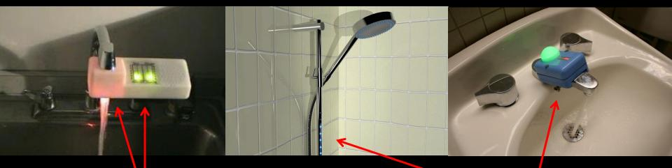
sensing and feedback unit co-located at fixture provides real-time feedback on water usage
