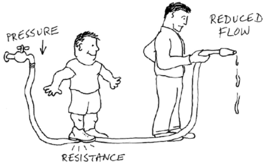
Figure 1-34. Larger resistance results in smaller flow—but if you increase the pressure, it may overcome the resistance and increase the flow.
