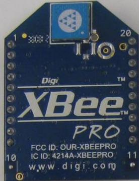
xbee wireless modem
