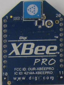
xbee wireless modem
