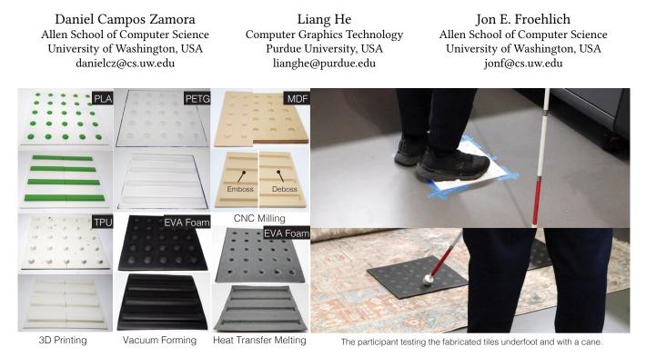
Figure 1: Samples of tactile surface indicators (TSIs) created via rapid prototyping methods (left) such as 3D printing, vacuum forming, CNC milling, and heat transfer melting–(right) which were evaluated through a qualitative study with a blind cane user to validate their tactile saliency as well as an O&M specialist.
