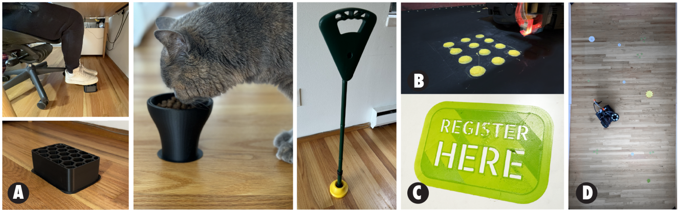
Figure 5: In situ 3D-printed examples by MobiPrint, including: (A) functional domestic objects like an ergonomic footrest, a raised pet feeding bowl, and a floor holder for a cane to prevent it from tipping over; (B) tactile navigation aids for people who are blind and low vision; (C) informational floor signage and graphics; (D) and decorative floor art.
