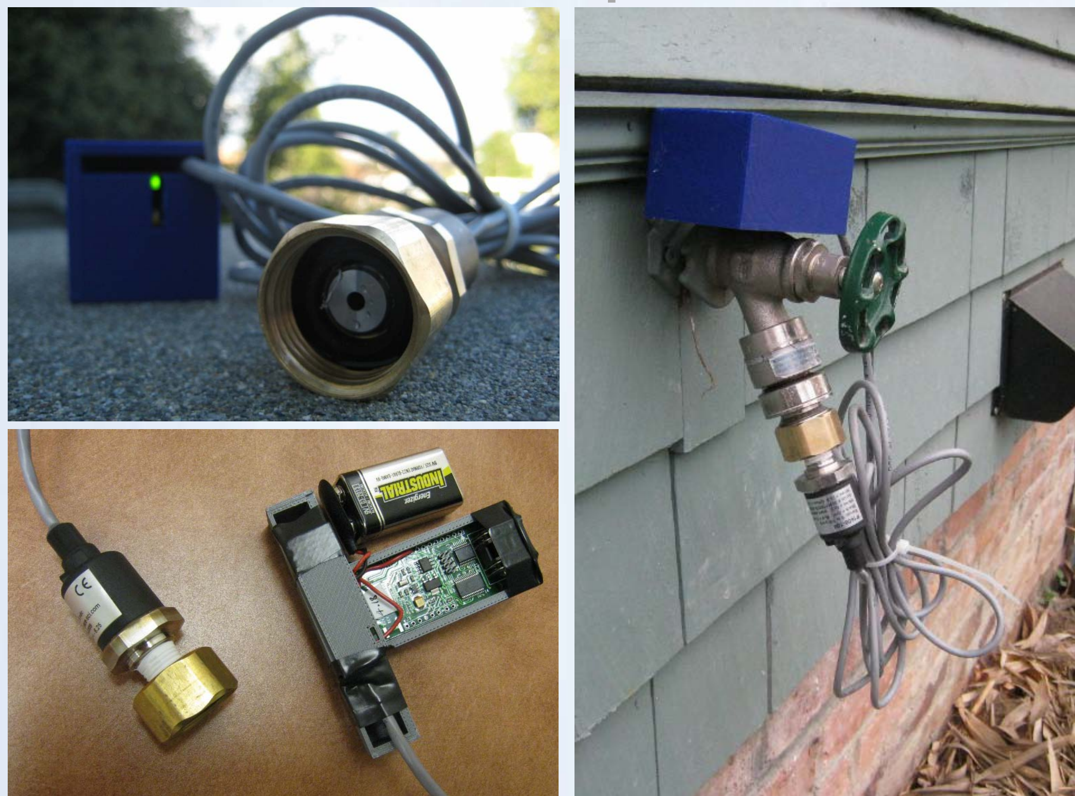
a single easy-to-install sensor continuously analyzes water pressure
