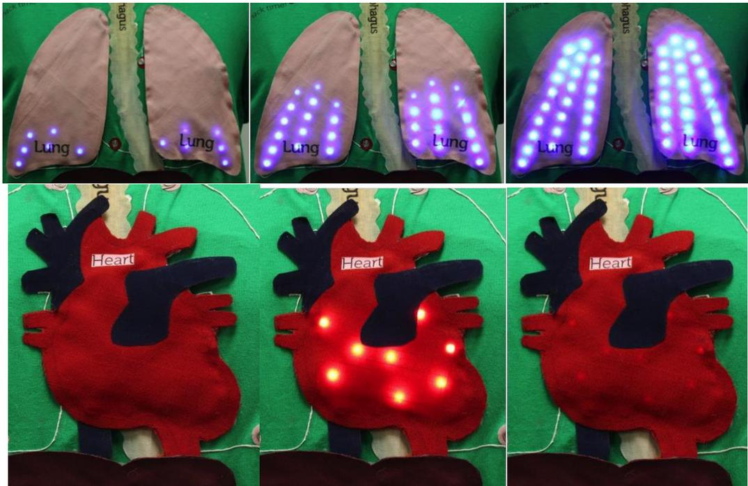
Figure 31: Lungs “inflate” when the LEDs fade on upwards (top left to right), and vice versa when they “deflate.” The LEDs in the heart abruptly turn on and fade off to mimic a heartbeat (bottom left to right).
