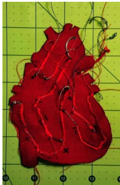
Figure 17: The heart contains LED pixels connected by conductive thread (silver thread), held down and protected by non-conductive thread (red thread).
