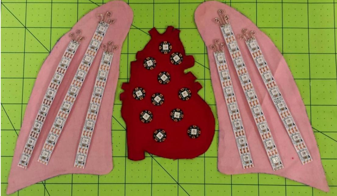
**Figure 18: Inside of the heart and lungs are LED pixels and strips, respectively.**
