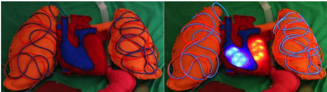
**Figure 10: On top, the heart and lungs in Prototype 1. On bottom, a close-up of the fabric heart (red and blue) with embedded LEDs and lungs (orange) with vein accents made of EL wire.**
