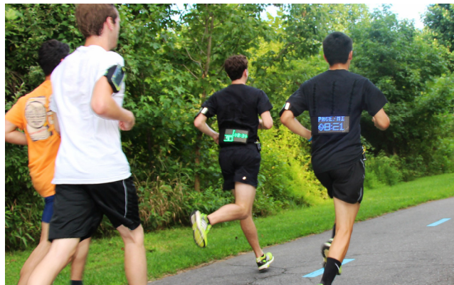
Figure 1: SFF visualizes real-time run-tracking information on shared, glanceable wearable displays to increase group awareness and fitness performance. See also the video in our supplementary materials.
