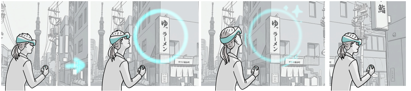
Figure 8: A walkthrough of LandmarkLens during navigation. As the user approaches an intersection, landmark highlights appear on the scene. A directional arrow prompts the user to look toward a highlight they haven’t yet noticed. Once the user gazes at the landmark, the circle pulses and fades, and the user proceeds to the next panorama.
