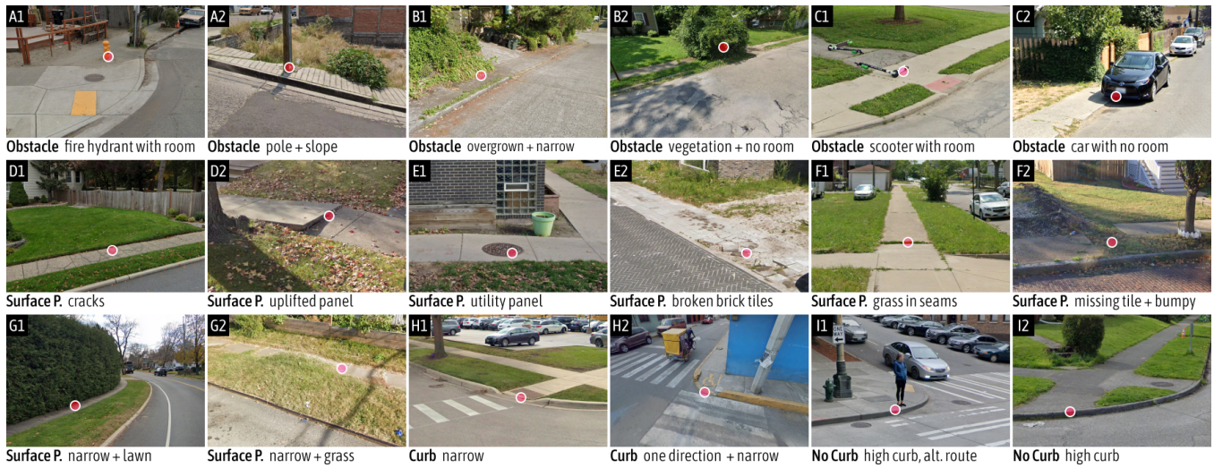
Figure 2: Our final image dataset consists of 52 images across nine categories, including fire hydrants + poles, overgrown vegetation, parked bikes/cars/scooters, cracks/height differences, bricks/cobblestone + utility panels, sand/gravel + grass, narrow, curb ramp, missing curb ramp . Above, we show two sample images from each category.
