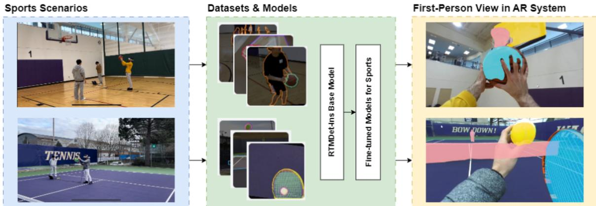
Figure 1: We contribute *ARSports*, a near real-time wearable stereo AR system to enhance sports playability for people with low vision composed of: (1) first-person basketball and tennis image datasets, which we manually collected and annotated; (2) accompanying fine-tuned instance segmentation models; and (3) a wearable AR research prototype that overlays visual augmentations (*i.e.*, instance segmentation masks) in an LV user’s residual field-of-view.
