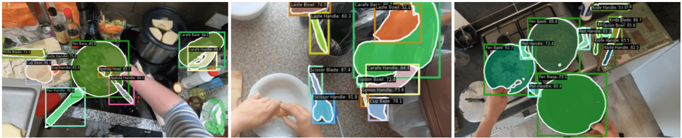
Figure 4: Example inferring results on images from the test subset of our dataset. These images demonstrate how the RTMDet-Ins-l-Cook identifies and segments graspable, safe areas—even in the presence of hands or other partial occlusions.
