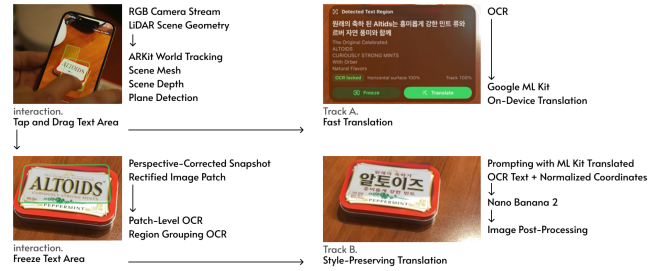
Figure 2: TranslateAR system pipeline. Tapping or dragging over a text region localizes it in 3D from RGB camera, LiDAR, ARKit tracking, and plane detection, yielding a fast semantic translation (Track A). Freezing the region then triggers an asynchronous style-preserving track (Track B) that rectifies, translates, and regenerates the patch before rendering it back.
