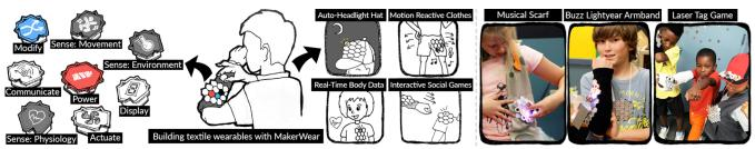
**Figure 1:** We introduce *MakerWear*, a new wearable construction kit for young children (K-6). By combining tangible, 'plug-and-play' electronic modules on a textile-integrated socket mesh, children can create a wide range of wearable designs from sound reactive clothes to interactive social games.
