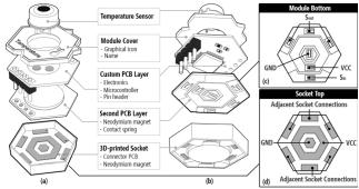
**Figure 3.** An exploded (a) top-down and (b) bottom-up view of an example MakerWear module and socket as well as overhead views of (c) module and (d) socket connector points. The contact springs ensure a robust connection.
