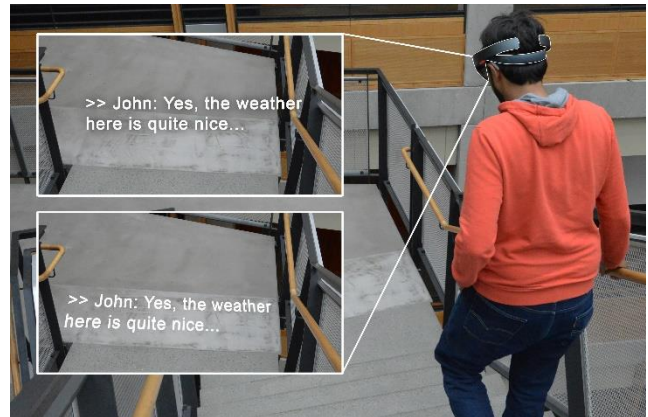
Figure 1: Illustrative image showing our lead author testing two different options for caption placement in our HoloLens prototype: (a) at a fixed distance from the eyes (here, 4m), or (b) automatically projected onto a surface (here, a floor).
