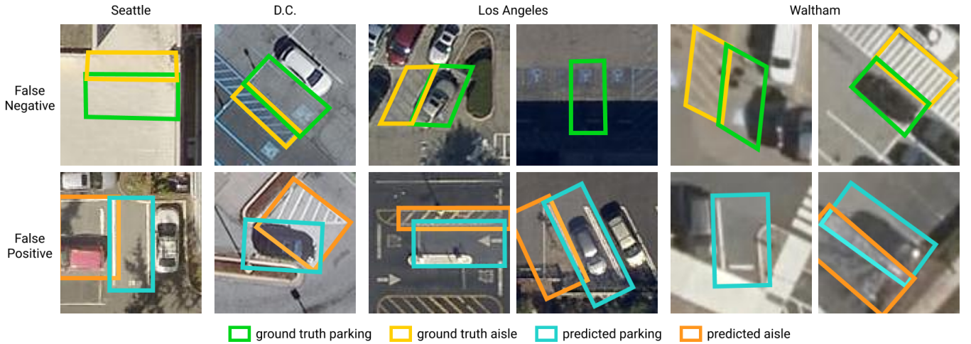
Figure 10: Example FNs and FPs for each evaluation region with ground truth annotations and predictions shown. We see similar error patterns as before; however, LA disability parking demarcations are often blue (rather than white or yellow) and more faded, resulting in lower contrast with the pavement. Waltham data is at a much lower resolution, resulting in blurriness.
