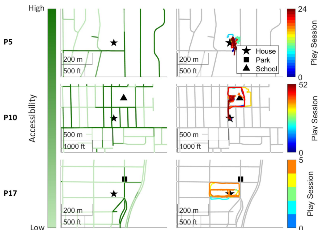
Figure 8. The accessibility scores for the sidewalks near each Participant's (P5, P10, P17) home on the left and the drive path of the participant on the right. Participants generally avoided driving on streets that were not accessible.
