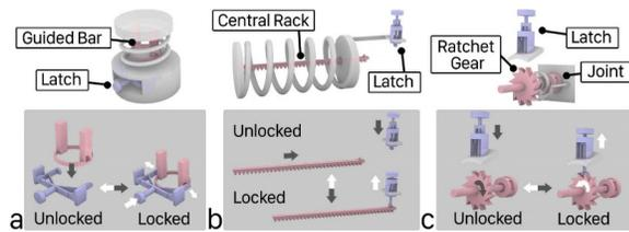
**Figure 3: Compliant lock mechanisms used in kinetic units: (a) guided bars and the compliant latch for the locking control of the helical spring in instant kinetic units, (b) the central rack and the compliant latch for the locking control of the helical spring in non-instant kinetic units, and (c) ratchet gear and compliant latch design for the locking control of the spiral spring.**
