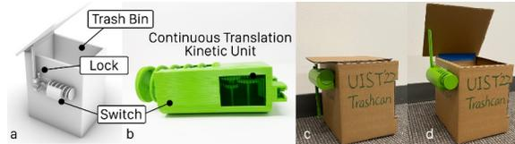
**Figure 13:** A continuous translation kinetic unit embedded switch is attached to a cardboard trash can: (a) the rendered 3D model of the switch and the trash can, (b) the printed switch, (c) the closed trash can with the switch attached and locked, and (d) opening the can's lid by unlocking the switch.
