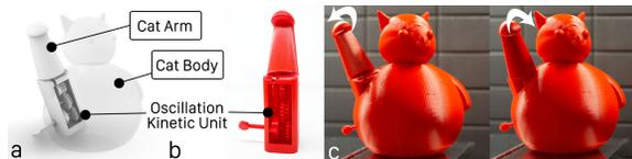
**Figure 16:** A battery-free Maneki Neko sculpture with an embedded oscillation kinetic unit: (a) the rendered model of the cat sculpture, (b) the printed kinetic unit-embedded arm, and (c) the waving arm in action.
