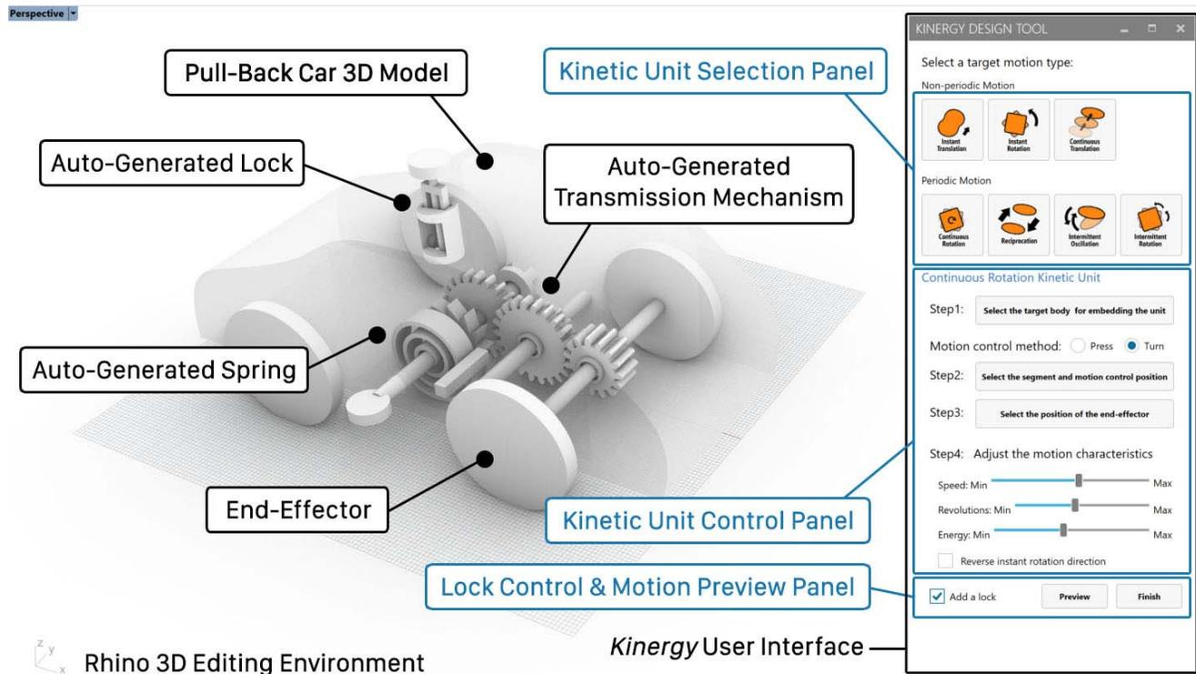
Figure 5: The user interface of *Kinergy* design tool.
