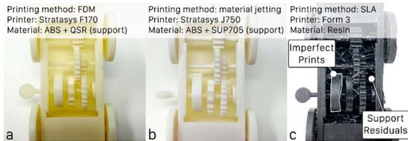
**Figure 10: The pull-back cars created with *Kinergy* are printed with various 3D printers and printing technologies: (a) industrial-level FDM 3D printing, (b) PolyJet 3D printing, and (c) SLA 3D printing.**
