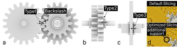
**Figure 9: Three types of tolerance identified as problematic for one-shot printing: (a) the gap between two mating gears, (b) the gap between a gear and its nearby spacer, and (c) the gap between a gear and its residing shaft. The 3D model is sliced in (d) an optimized orientation and the slicing settings are curated to create clean part contours for intermating elements.**
