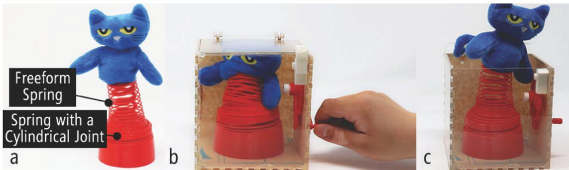
Figure 4.17: A jack-in-the-box spring mechanism generated by *Ondulé*: (a) two spring designs are embedded; (b) the cat can be fully compressed and locked inside a laser-cut box; and (c) the cat pops out following a path as a surprise.
