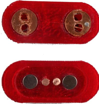
Figure 35: The front (top) and back (bottom) of the “snap” connection interface.
