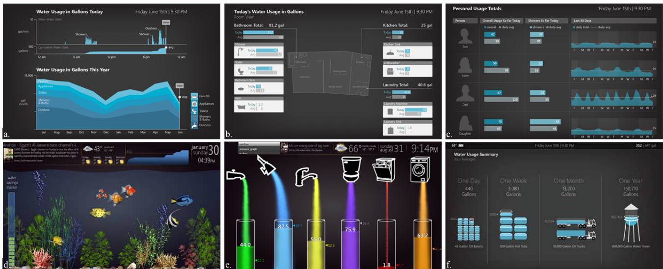
Figure 3: Six of the design probes: (a) the Time-Series view shows water usage over the current day and year; (b) the Spatial view uses a floorplan to show room-level and fixture-level usage; (c) the Per-Occupant view shows water usage broken down by the current day and past month; (d) the Aquatic Ecosystem explores the use of ambient game elements to motivate water savings; (e) the Rainflow view is a stylized, more ambient version of the fixture category base bar graph design; (f) one of the Metaphorical Unit views, which uses common objects to depict average daily, weekly, monthly, and yearly usage. The top three design probes were evaluated in the survey; all were evaluated in the interviews.
