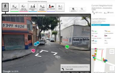
Fig. 1: The Project Sidewalk labeling interface (in English) showing a labeled street scene in Azcapotzalco, MX with a curb ramp (green label), a missing curb ramp (red), and a tree and pole in the middle of a narrow sidewalk (blue).
