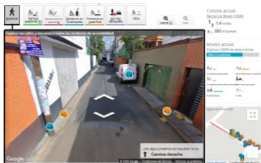
Fig. 2: The Project Sidewalk interface (in Spanish) showing narrow sidewalks with surface problems (orange labels) and physical obstacles (blue labels) in Azcapotzalco, MX. Screenshot from Twitter @Gari01234 .
