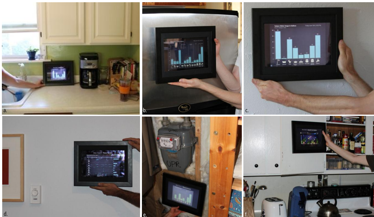
Figure 9.18: Preferred display locations in (a) H5, (b) H4, (c) H1, (d) H10, (e) H6, and (f) H8. Most selected a highly visible, easily glanceable location (e.g., H5 and H4 selected the kitchen and H1 and H10 selected hallways). H6 and H8, however, preferred behind the cupboard or in a closet next to the gas meter.
