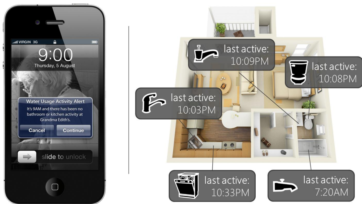
Figure 10.5: HydroSense can be used for applications beyond eco-feedback. For example, in this figure, disaggregated water usage is used in an envisioned assistive care application to automatically alert care givers to a potentially health threatening situation.
