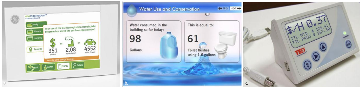
Figure 4.5: (a) General Electric’s Ecomagination display uses cartoonish iconography to display energy consumption values in terms of dollars, tons of CO 2 and miles driven. (b) The Lucid Design Group Building Dashboard display uses metaphors in terms of gallon jugs and toilet flushes to convey water usage. (c) The Energy Detective (TED) can be set to display electricity usage in terms of cost or kWh; here the display is showing cost/hour.
