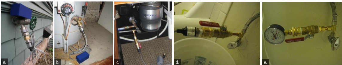
Figure 7.1: HydroSense is a pressure-based sensing solution that disaggregates water usage at the fixture level from a single installation point. HydroSense uses a digital pressure sensor that can be installed onto (a) an exterior hose bib or (b) water heater drain valve in the same way that one would attach a garden hose. If these installation points are not available, HydroSense can also be installed at the 3/8" hose connection points of toilets (not shown), (c) kitchen sinks or (d) bathroom sinks. (e) An analog pressure gauge shown for comparison.
