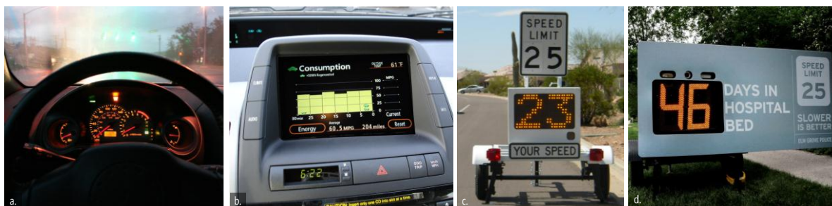
Figure 1.3: Different ways of presenting feedback about driving behavior: (a) the traditional dashboard, (b) the Toyota Prius dashboard, (c) a vehicle activated sign that displays sensed speeds of oncoming traffic, and (d) a clever variation on (c) that changes the currently sensed speed into a persuasive message. Each presentation can have a different impact on behavior.
