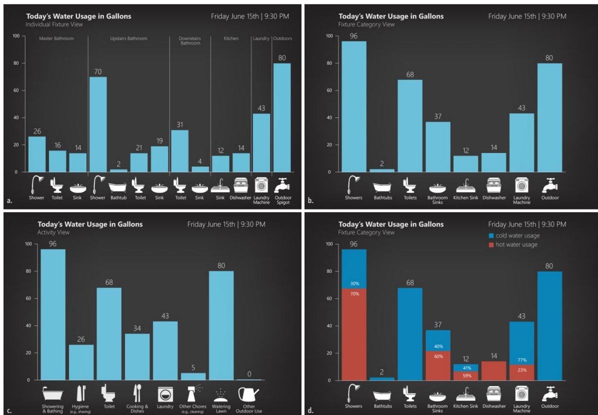
Figure 9.2: The four Data Granularity views: the Individual Fixture View , the Fixture Category View , the Activity View , and the Hot/Cold Breakdown View .
