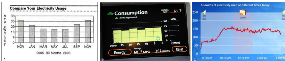
Figure 4.3: Different time windows: (a) A Seattle Public Utility electricity bill shows a bar graph of electricity usage over the past year (including the current month). (b) The Toyota Prius dashboard display shows mileage and regeneration information for the last 30 minutes. (c) Lucid Design Group’s building dashboard shows electricity use, in this case, over the course of a day.
