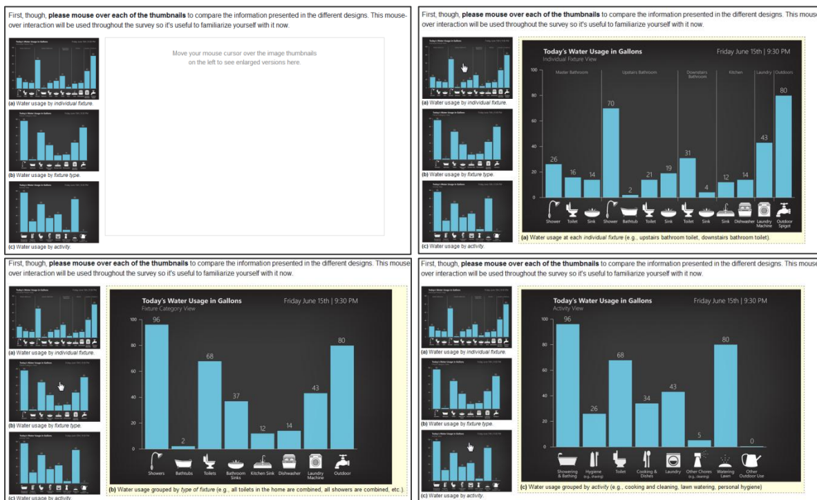
Figure 9.14: Using custom CSS and HTML code in SurveyGizmo, we were able to create mouseover interactions of thumbnails, which showed enlarged versions of the moused-over design in the middle of the browser window. This allowed respondents to quickly compare and contrast the different designs presented on each page.
