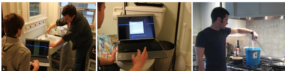
Figure 7.9: Collecting controlled experimental water usage trial data using the HydroSense Logger tool visible in (a) and (b). In (c), collecting flow rate data in addition to logging sensed pressure.
