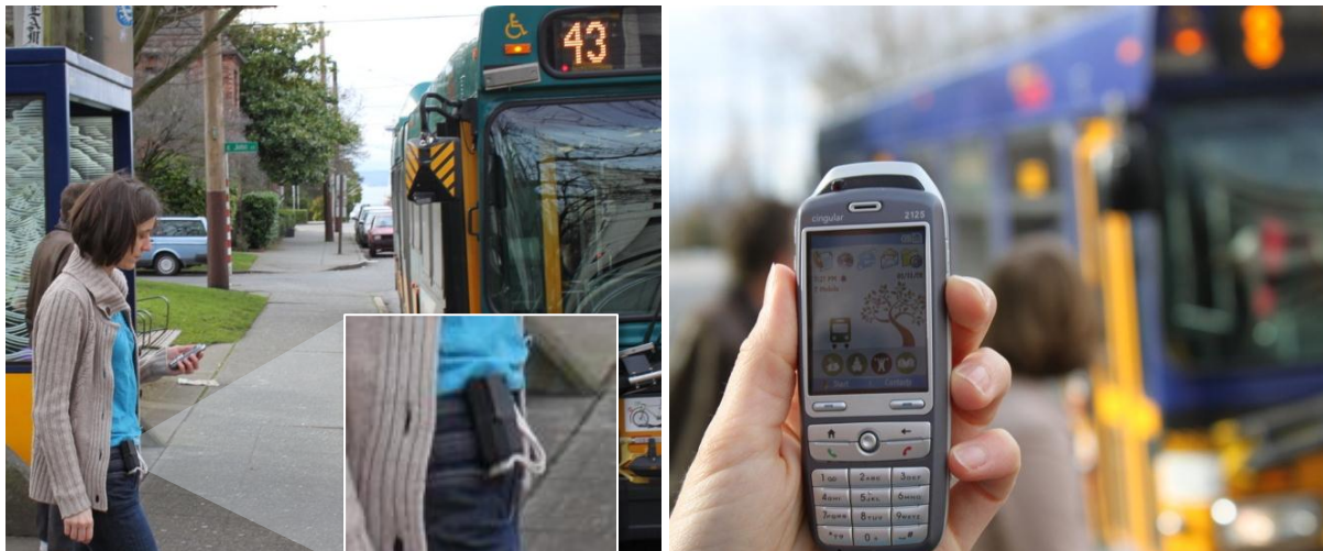
Figure 5.1: The UbiGreen Transportation Display semi-automatically senses routine travel behavior such as walking, bicycling, and taking the bus and visualizes this information on the background (“wallpaper”) of the mobile phone in order to promote awareness and support green transportation habits.
