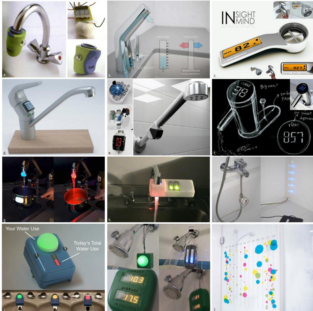
Figure 2.4: Thus far, most water-based eco-feedback systems have been designed to sense and feedback water usage at the point-of-consumption . The top two rows are design sketches/conceptions created by industrial designers while the bottom two rows are actual systems built and evaluated by HCI researchers. Starting from the top-left: (a) Squirr by Meghana Vaidyanathan (Lockton, 2007) is aimed at children aged 3 to 6. (b) In-Formed by Nadeen Haidary redirects a small portion of water to a glass chamber, which acts as a bar graph tracking current usage. (c) Insight/Inmind by Adam Kereliuk (Morell, 2007) uses a backlit LCD display to show how much water usage a faucet/shower has used by day, week or month; the next three designs are similar: (d) TapMeter by Henry Ellis-Paul, (e) Domestic Water Meter by Viktor Legin, (f) iSave by Yu Guogun (Morell, 2007). (g) HeatSink (Arroyo et al. , 2005) illuminates water according to temperature while (h) WaterBot (Arroyo et al. , 2005) offers continuous feedback via visual and auditory cues. (i) The Show-Me shower display by Kappel and Grechenig (2009) illuminates a string of LEDs according to usage. (j) and (k) show various UpStream prototypes for faucets and showers by Kuznetsov and Paulos (2010). (l) The Shower Calendar by Laschke et al. (2011) uses a projected display on a shower curtain to show shower usage amounts over time (colors represent people; larger dots mean less water usage during that shower).
