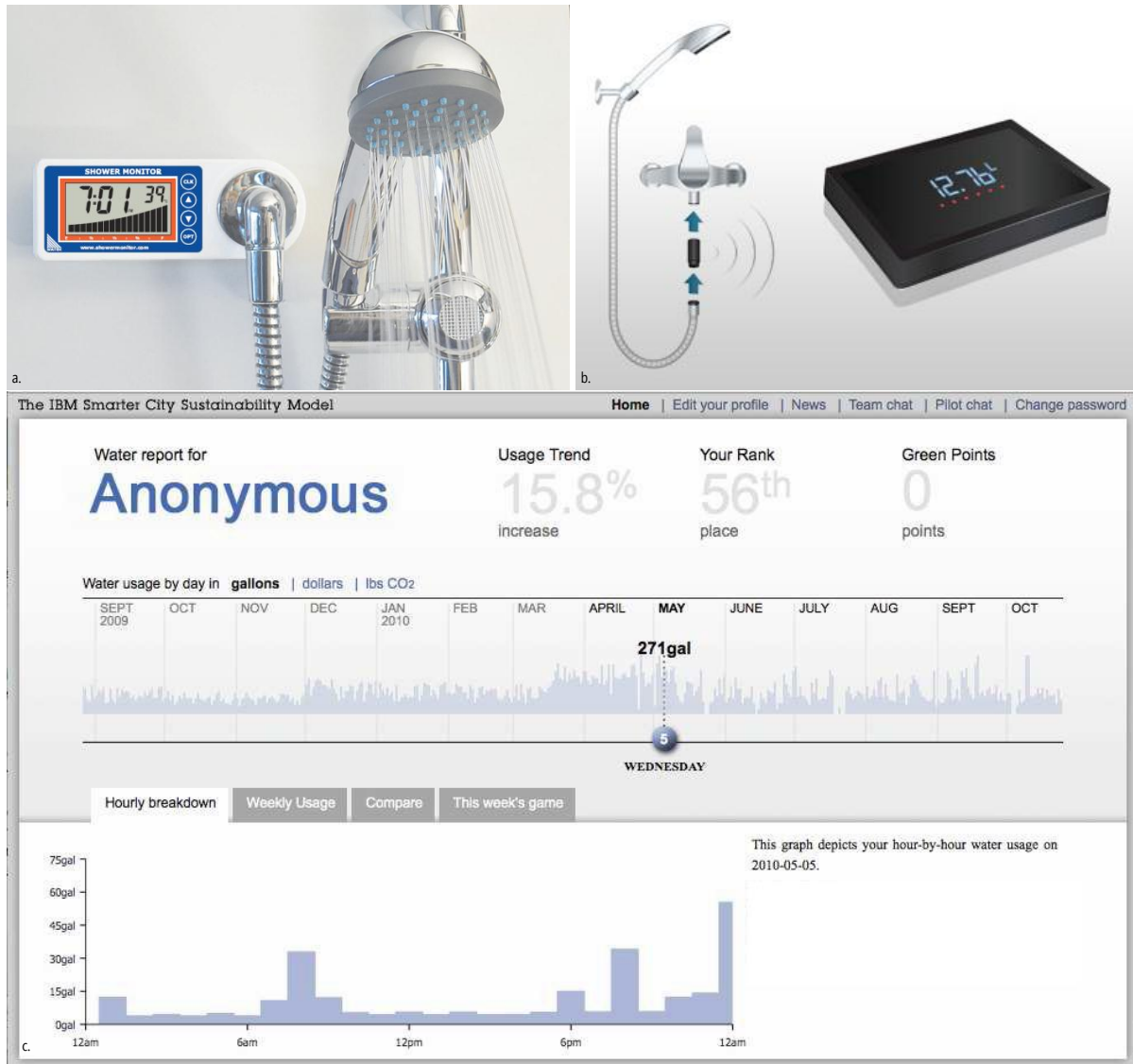
Figure 2.5: Three commercial eco-feedback systems for water: (a) The Shower Monitor by Waitek starts with a full “progress-bar” that decreases according to sensed flow rate and water temperature. After a preset amount of water has been used, a beeper alarm sounds (see Willis et al. , 2010). (b) The start-up company Amphiro has recently pilot tested their miniaturized smart meters with wirelessly connected displays; however, little information exists on the design of their system (see Staake et al. , 2011). (c) The IBM Smarter City Water Pilot (Naphade et al. , 2011) is an online website for smart meter water data that was deployed to 151 households over a 9-week period. These three designs were also evaluated in behavioral studies, see Table 2.3.
