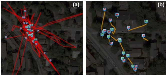
Figure 4. (a) 34 garbage trips were created by GPS location drift over a three day period while this driver's vehicle was parked outside his house. (b) These garbage trips were transformed to intermediate centroid based trips (shown in orange), which are less than 0.1 miles in length and therefore are filtered out of our dataset.
