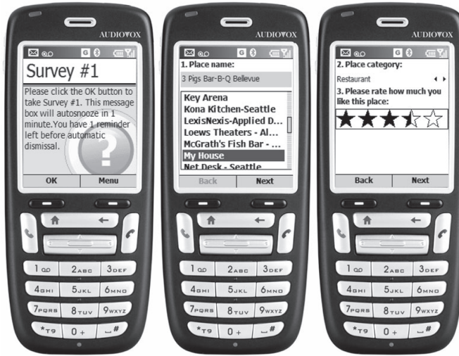
FIGURE 3 ESM questions on the SmartPhone Audiovox SMT 5600. Shown are examples of the survey prompt screen (left), text entry auto-completion (middle), and rating scale (right) questions used in the “voting with your feet” study.
