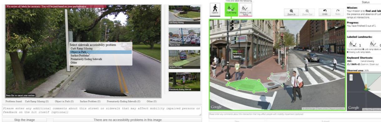
Figure 8. Our custom image labeling tools on web browsers: (a) The early version of the interface, which lets a user mark the location of the sidewalk problem and categorize the problem type (e.g., an obstacle in a path) on a static GSV images [6]; (b) The labeling interface from our most recent work [10], which allows a user to adjust the camera angle (pan and zoom) and search for and label accessibility attributes in GSV.
