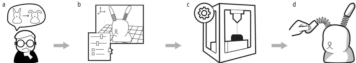
Figure 1: Proposed workflow of making deformable 3D-printed objects – (a) ideating possible deformation behaviors; (b) designing and simulating deformable parts in our CAD tool; (c) fabricating with modified g-code and printer; (d) validating in the real world.
